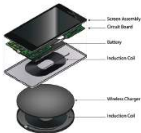
Fig 2.3.5: Wireless charging technology
